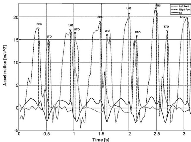
**Fig. 3 – Superimposition of typical anterior-posterior acceleration signals (subject #2), from the sensor on L5 (solid line), and from the sensors on the forefeet (dash-dotted for the right and dotted for the left) along a few steps. The timing of the gait-related events as assumed in most of the previous literature is also shown (dashed vertical lines,): right foot heel strike (RHS) and toe-off (RTO), left foot heel strike (LHS) and toe-off (LTO).**
